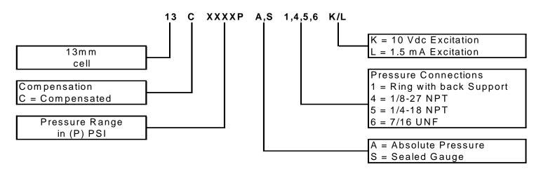
For example: Part #13C3000PS4K = 13 mm Cell, Compensated, 3000 psi, Sealed Gauge, 1/8NPT Port, with 10 Vdc excitation.
