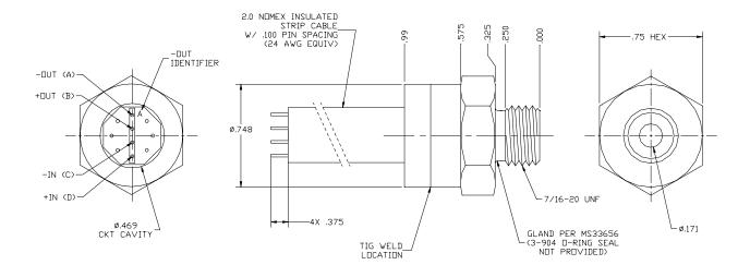
Note1: Non-concentricity effects at the diaphragm weld area may cause run out of up to  $\pm 0.006$ " between the upper and lower portions of the sensor body. (It is recommended to use a counter bore in the mating bore used with this device to allow for this non-concentricity.)
