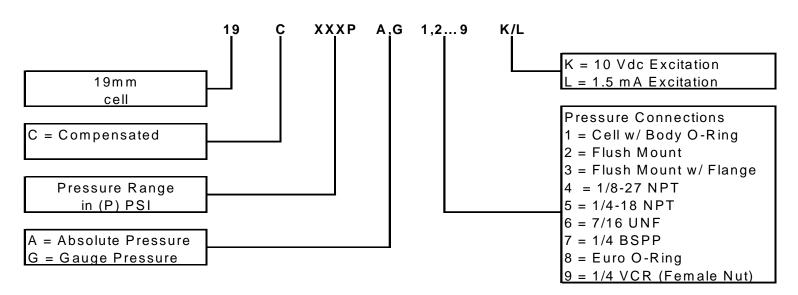
For example: Part #19C100PA4K = 19 mm Cell, Compensated, 100 psi, Absolute, 1/8NPT Port, with 10 Vdc excitation.
